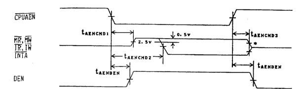
\* Measured at the point where output voltage changes 0.5V.
