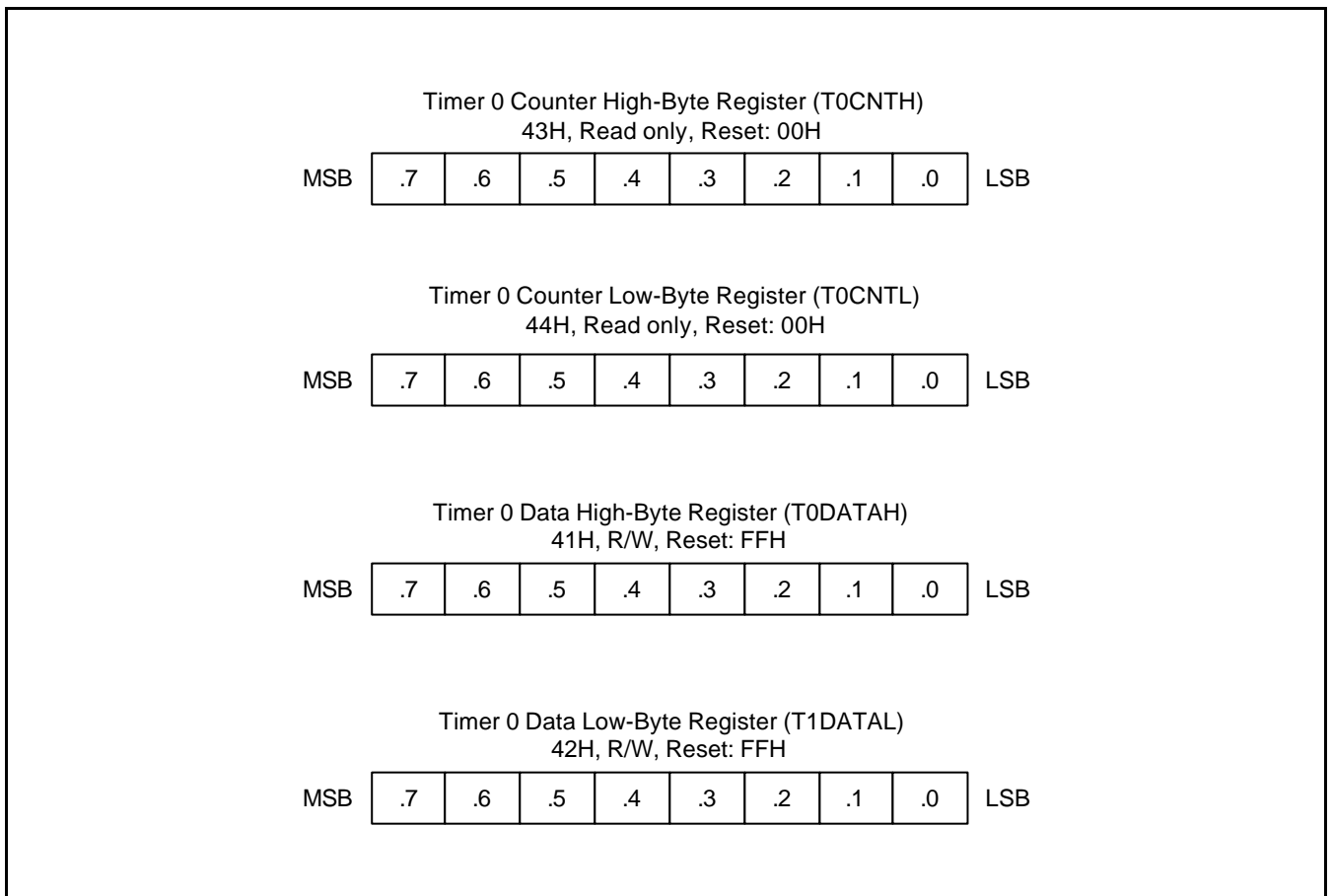
Figure 13-3. Timer 0 Counter and Data Register (T0CNTH/L, T0DATAH/L)
