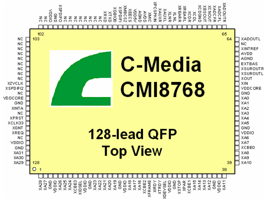
Figure 5. Top View of CMI8768
