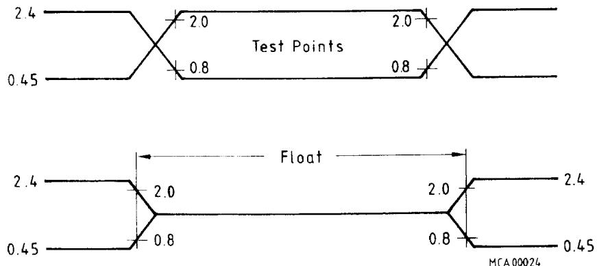
AC testing inputs are driven at 2.4 V for a logic "1" and at 0.45 V for a logic "0".
