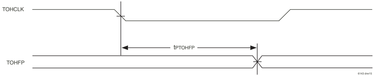
Figure 50 Transmit Overhead Output Timing
