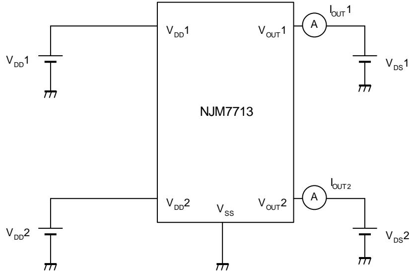
③ Pch OUTPUT CURRENT TEST CIRCUIT
