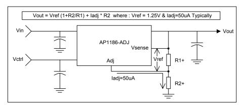
The AP1186-ADJ keeps a constant 1.25V between the Vsense pin and the Adj pin. By placing a resistor R1 across these two pins and connecting the Vsense ans Vout pin together, a constant current flows through R1, adding to the ladj current and into the R2 resistor producing a voltage equal to the (1.25/R1)\*R2 + ladj\*R2. This voltage is then added to the 1.25V to set the output voltage. This is summarized in the above equation.
