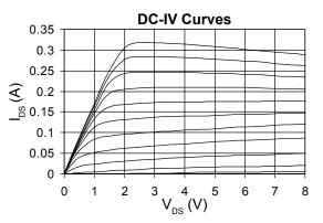
$V_{GS}$  = -2.0 to 0V, 0.2V steps T=25°C
