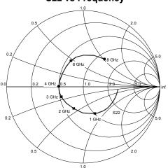
Note: S-parameters are de-embedded to the device leads with  $Z_s = Z_L = 50\Omega$ . The data represents typical performace of the device. De-embedded s-parameters can be downloaded from our website (www.sirenza.com).
