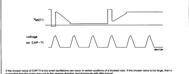
is possible that the motor may run in the reverse direction (synchronously with little torque).
