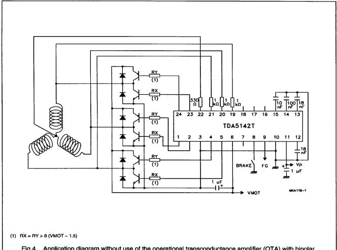
Fig.4 Application diagram without use of the operational transconductance amplifier (OTA) with bipolar power transistors.
