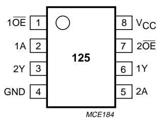
Fig.1 Pin configuration.
